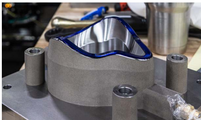
Figure 2: Researchers at ORNL's MDF developed a reusable face mask prototype with injection molding that will enable industry to rapidly manufacture masks. The injection-molded reusable mask includes five parts, and with five sets of tools, industry can potentially make 300,000 reusable masks per week. Credit: Carlos Jones/ORNL, U.S. Dept. of Energy.
