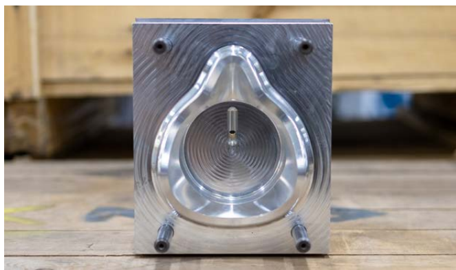
Figure 2: Researchers at ORNL's MDF developed a reusable face mask prototype with injection molding that will enable industry to rapidly manufacture masks. The injection-molded reusable mask includes five parts, and with five sets of tools, industry can potentially make 300,000 reusable masks per week. Credit: Carlos Jones/ORNL, U.S. Dept. of Energy.
