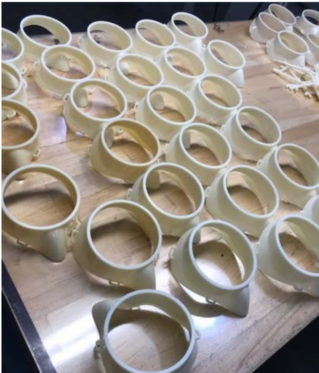
Figure 3: ORNL is designing reusable face masks using the lab's advanced manufacturing facilities. Credit: ORNL, U.S. Dept. of Energy.
